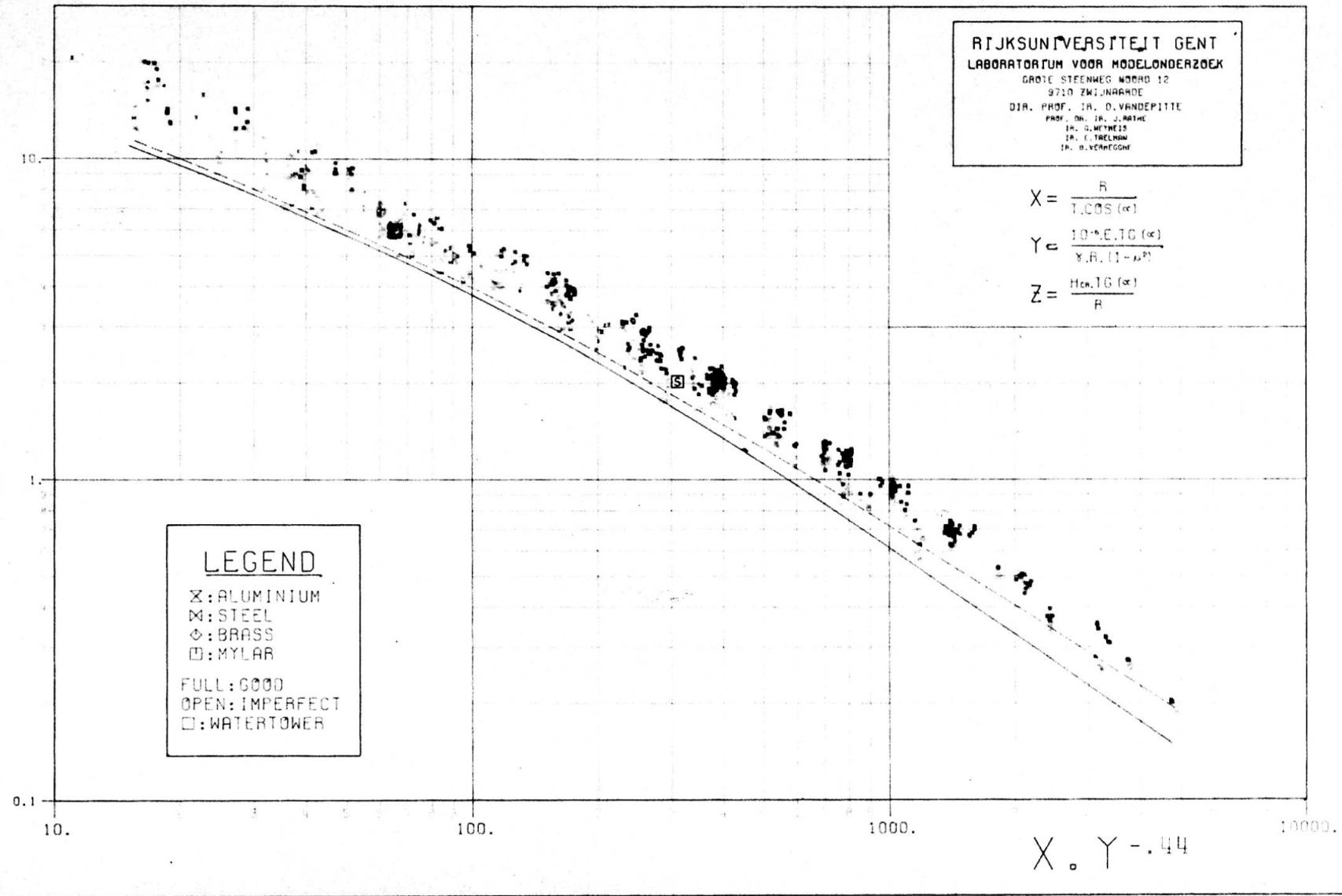
shown in figure 2. This figure illustrates the relatively small scatter of the test data, small, that is, for buckling tests on shells. Note should be taken, however, of the fact that, owing to the representation of the ordinates to a logarithmic scale, the scatter is wider than one might infer from a glance at the diagram.
