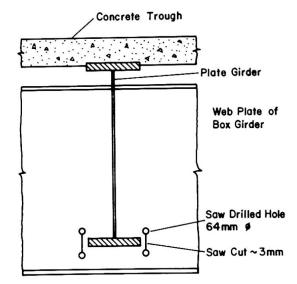
Fig. 6a Retrofitted Box Side Plate
