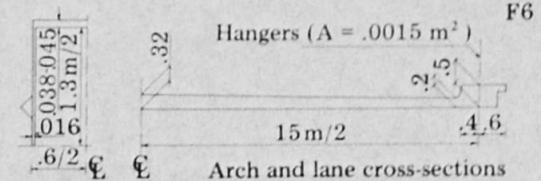
When many hangers relax bending moments in the chords are bigger than when the span acts like a truss. The normal forces in the chords, however, are smaller than maximum because the live load is only on part of the span.
