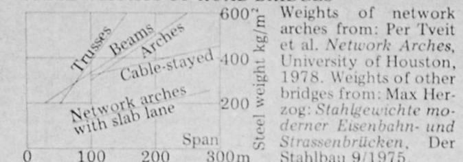
Weights of network arches from: Per Tveit et al. *Network Arches*, University of Houston, 1978. Weights of other bridges from: Max Herzog: *Stahlgewichte moderner Eisenbahn- und Strassenbrücken*, Der Stahlbau 9/1975.
