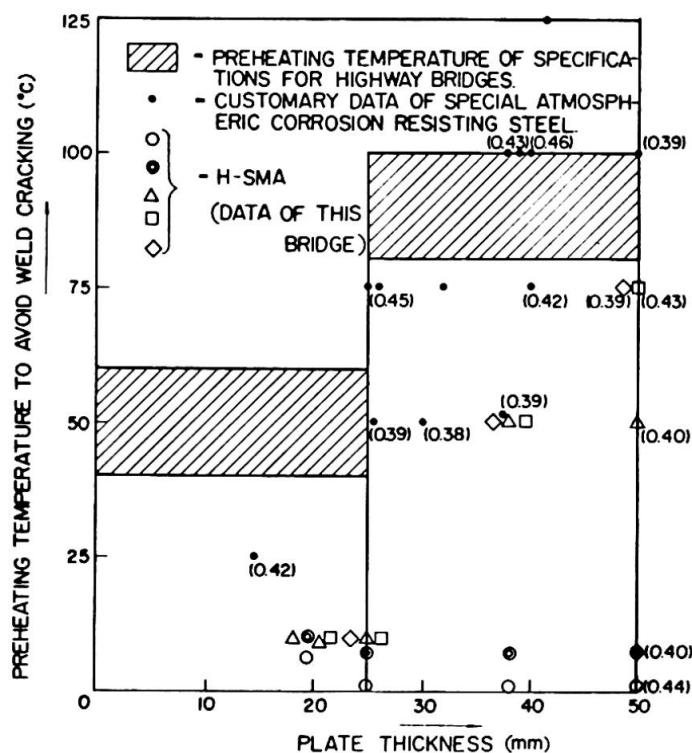
FIG.2 Y-SLIT CRACKING TEST RESULTS
