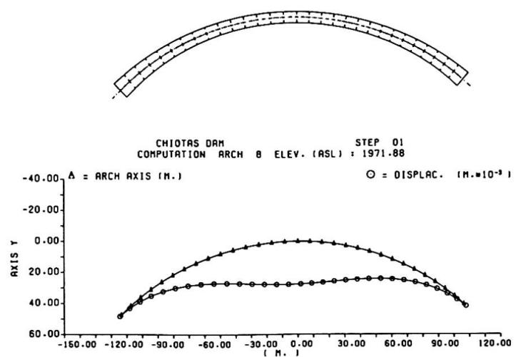
Fig.5 Deformation of central fiber of an arch.
