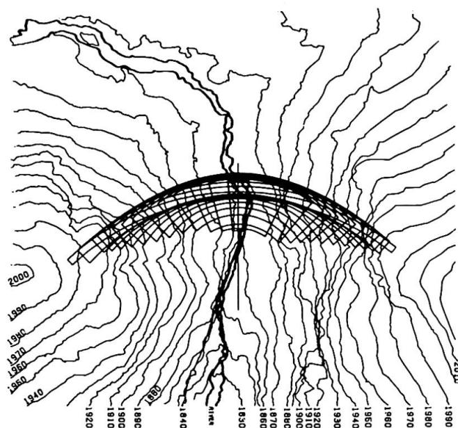
Fig.2 Valley contours and superposed arches of Chiota's dam.
