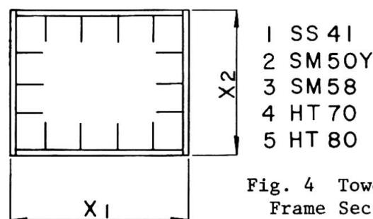
Fig. 4 Tower Frame Section
