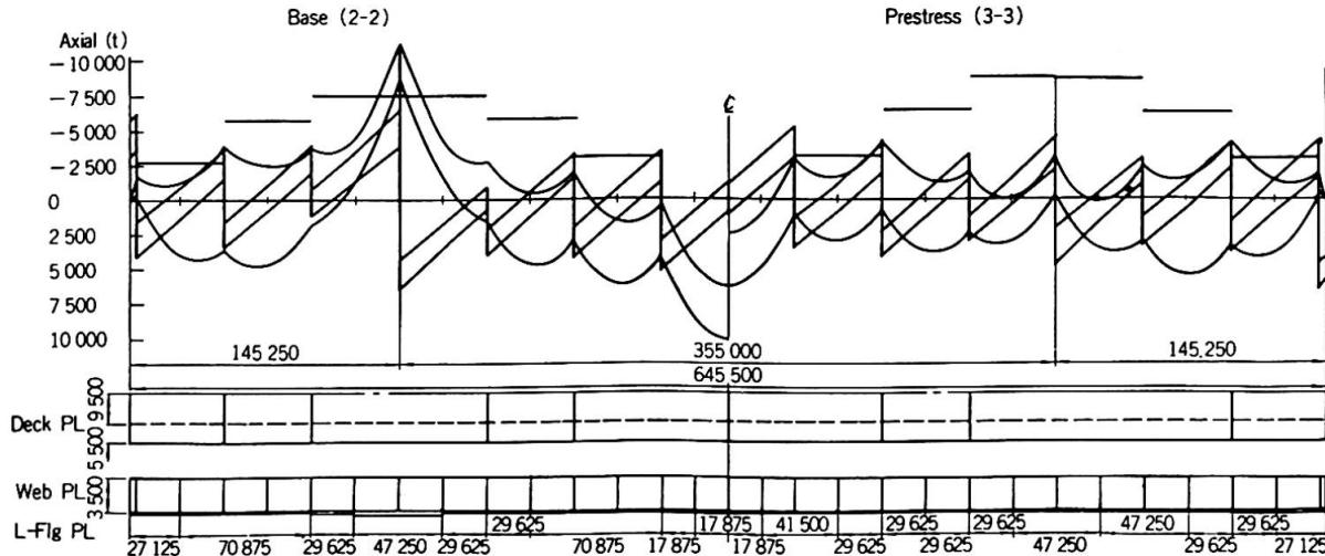
Fig. 7 Section Force Diagram and Basic Girder Section
