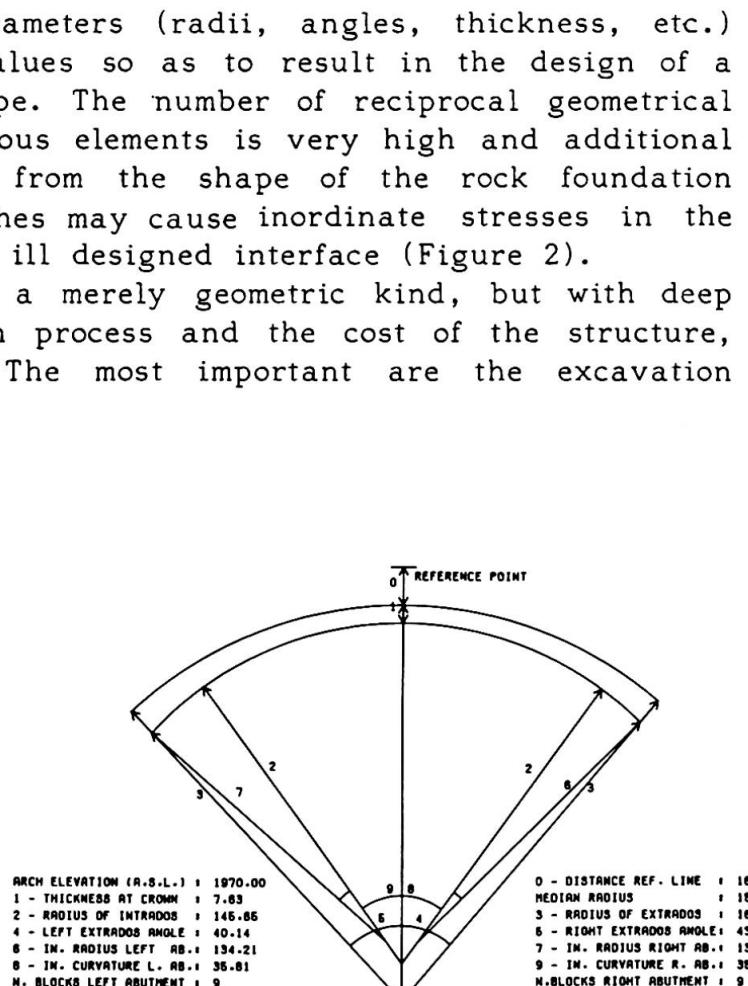
Fig.3 Geometrical input data of an arch.
