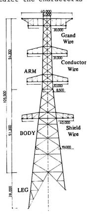
Fig. 1 Example of ultra high voltage electrical transmission towers (mm)
