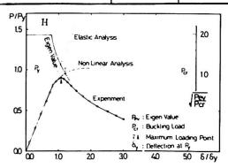
Fig. 9 Prediction of buckling load of leg
