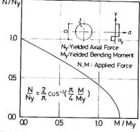
Fig. 3 Moment-axial force interaction curve
