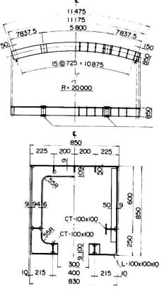
Fig. 3 Dimensions of guideway model (JIS-SS4I)
