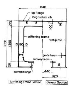
Fig. 2 Cross-section of guideway
