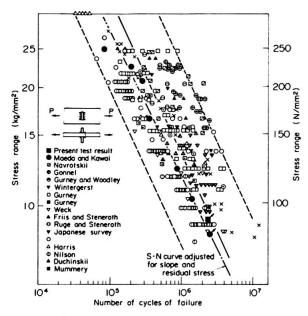
Fig. 8 S-N curve for transverse non-load-carrying fillet welded joints
