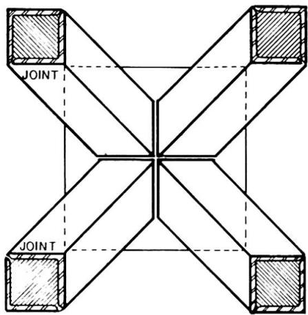
Fig. 3 Upward View of an Intermediate Node (Sketch)
