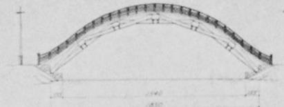
Dimensions of the bridge, as estimated from studies of writings by different authors in Sung dynasty are shown on picture. Calculated by electronic computer, the timber arch segment is about 30 cm in diameter. The total material required is 0.423  $\text{m}^3$ , including hand rails and deck plants.
