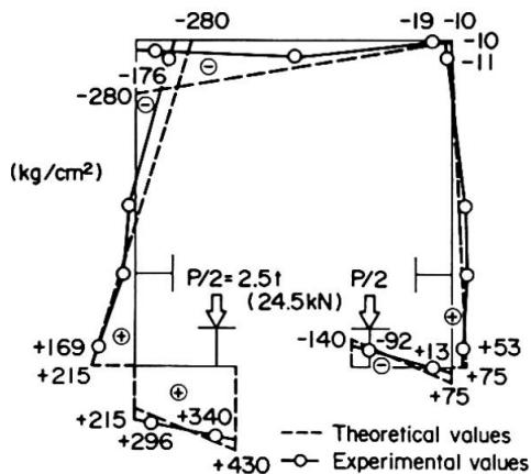
Fig. 6 Distribution of longitudinal stresses at mid-span cross-section
