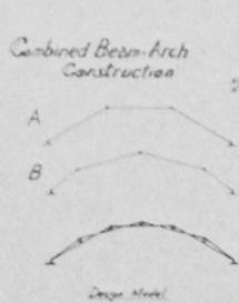
The bridge structure consists of two basic systems, system A and B. Both systems are unstable structures, as they are held together by non-connection with timber strips.
