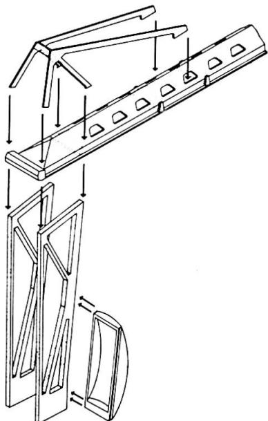
Fig.12. Axonometric view of the precast elements
