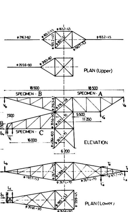
Fig. 6 Specimens of arm (mm)
