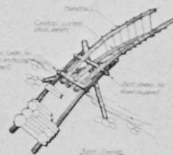
The construction of the bridge is shown on the picture. Longitudinal beams are inserted in the mortise on each bank, and counteracted out to the river. The gap between two counteracts is then connected by another beam. Binding the counteracts beams firmly with timber strips, the Bow Bow bridge is finally completed.
