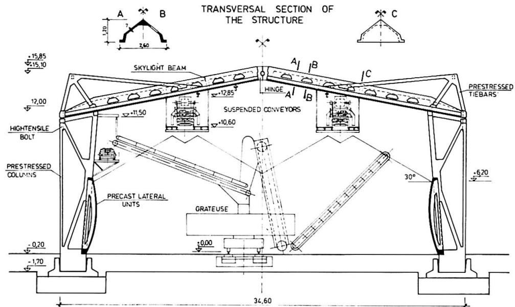
Fig.11. Cross section of the depot structure
