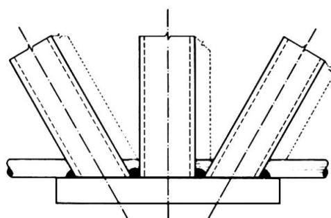
Fig. 6 Detail of a Lower Bearing Node (Sketch)
