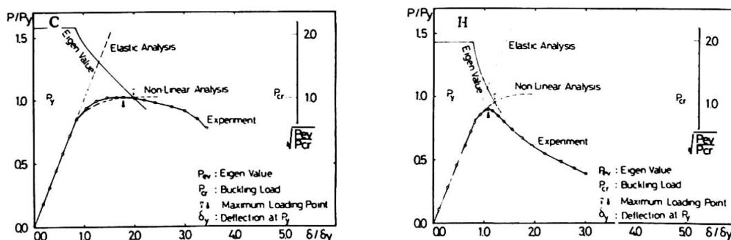
Fig. 9 Prediction of buckling load of leg
