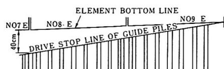
Fig. 10 Pile arrangement in the axial direction
