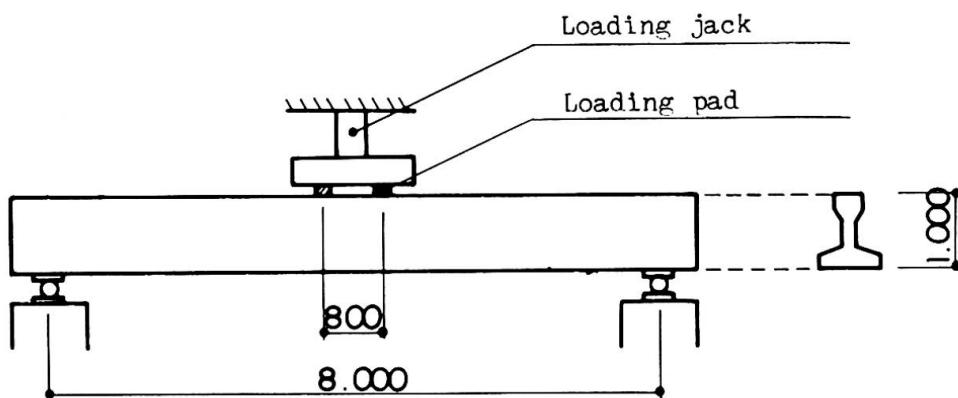
Fig.3 Loading method
