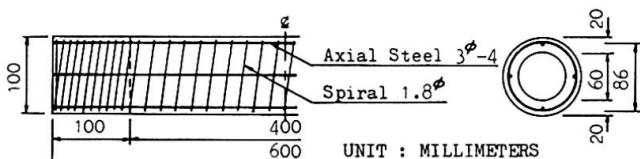
Fig. 1 Details of Model Pile
