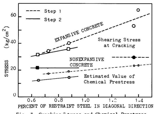
Fig. 3 Cracking Stress and Chemical Prestress
