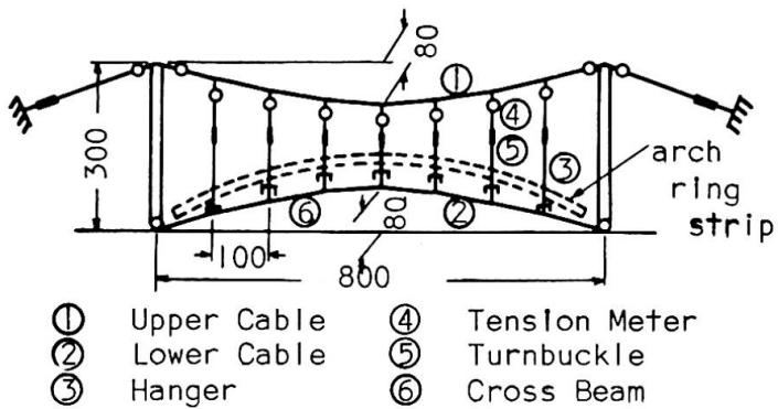
Fig.2 Pretensioned Cable Truss
