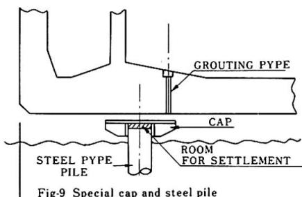
Fig. 9 Special cap and steel pile
