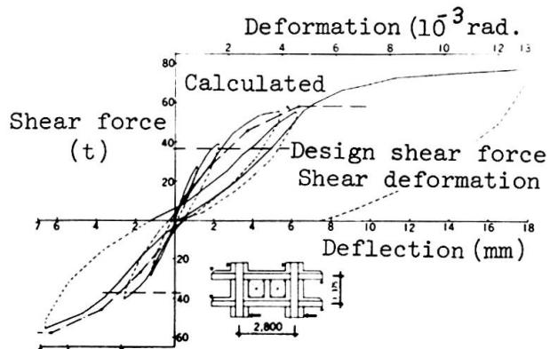
Fig. 5 Load-deflection curve of frame specimen
