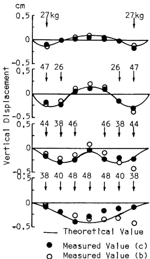
Fig.7 Vertical Displacement of Cross Beam (b), (c)
