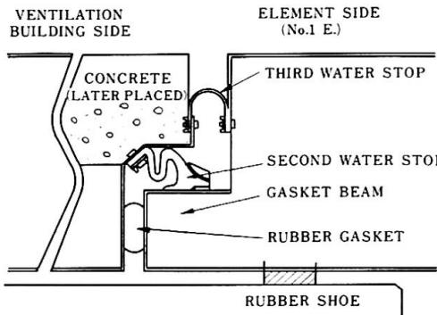
Fig.6 Details of the first joint
