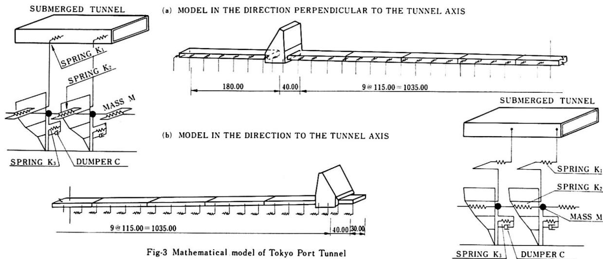
Responses in two directions were calculated mainly by using EL Centro NS 1940 and Aomori NS 1968 (Off-Tokachi Earthquake) records as in-put seismic waves, the latter having comparably longer period when compared with the former. As a result of calculations, the followings were learned:
