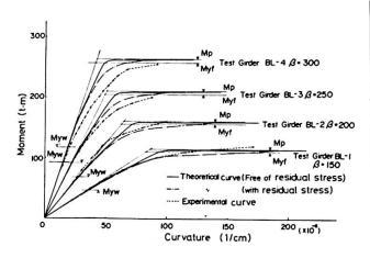
Fig. 1. Moment v.s. curvature curve
