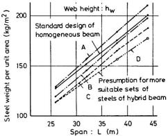
Fig. 6. Weight comparison of hybrid composite girders with homogeneous ones
