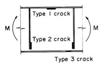
Fig. 2. Types of fatigue cracks under pure bending
