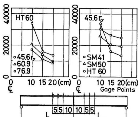
Fig.5 Strain Distribution
