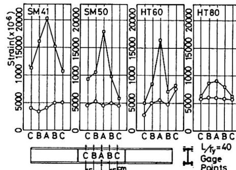
Fig.4 Strain Distribution
