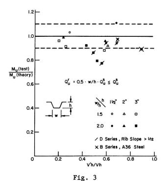
All of the test beams sustained maximum deflections between 8 and 22 in. (203 to 560 mm). These deflections correspond to more than ten times the deflection at working load in all but two cases. Such large deflections were permitted by the formation of a plastic hinge near the midspan in all of the beams. The formation of these plastic hinges which produced the deflects.4) sired ductility could only have been possible with a ductile shear connection.
