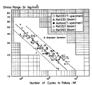
Fig. 7 Comparison of previous work on Type 3 crack with this study
