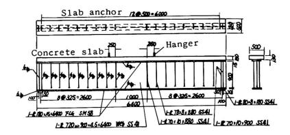
Fig. 4 Bending Test Specimen with Slab (Type GS)
