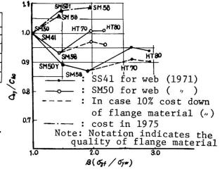
Fig. 1 Relations between  $\beta$  and  $C_{hy}/C_{ho}$ strength steel as HT80 is reduced in future, this type of girder will be superior
