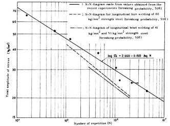
Fig. 10 S-N Diagram of Hybrid Material
