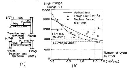
Fig. 3. S-N curves for Type 2 crack
