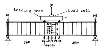
Fig. 5 Loading method for Bending Test
