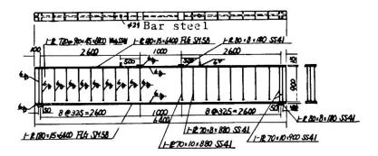
Fig. 3 Bending Test Specimen (Type G)
