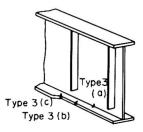
Fig. 1 Types of fatigue cracks under pure bending
