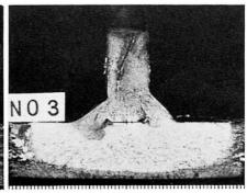
Fig. 4 Fracture surface (from worm-hole)
