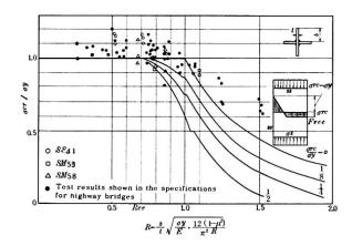
Fig. 8 Buckling Curve for Compression Hybrid Column
