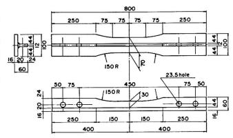
Fig. 2 Details of test specimen
