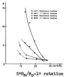
capacity Fig.2.9 Relationships between R and  $(b/t)\sqrt{\sigma_v}$
