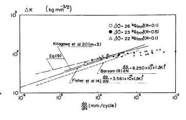
Fig. 10 Fatigue crack-growth rate
