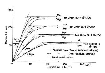
Fig. 1. Moment v.s. curvature curve
