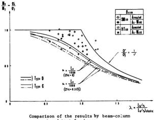
Comparison of the results by beam-column approach and test for beams  $% \left\{ 1,2,\ldots ,n\right\}$
