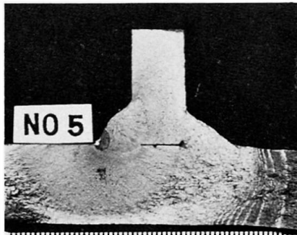
Fig. 5 Fracture surface (from under-cut)
