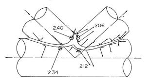
Fig. 6 Principal Stresses in Tubular K-Joint
