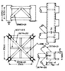
Fig. 2 Full-Scale Joint Specimen
