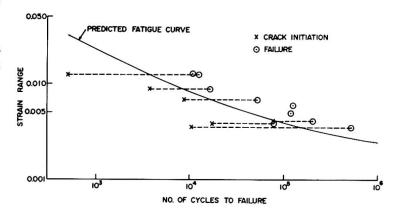
Fig. 7 Fatigue Test results on Model Joints
