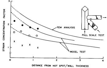
Fig. 4 Strain Distribution in Corner Joint
