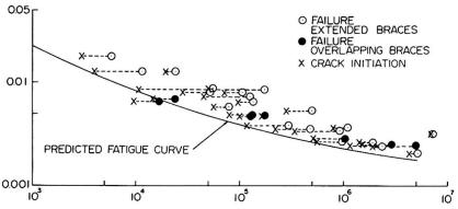
Fig. 8 Fatigue Test Results on Tubular K-Joints
