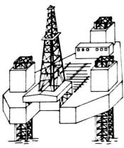
Fig. 1 Offshore Jack-Up Platform
