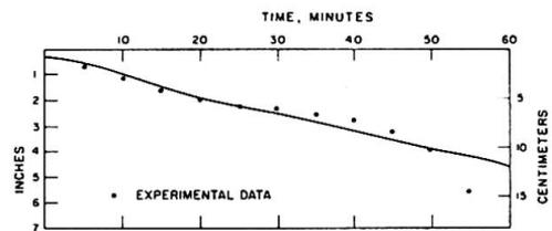
FIG. 7 COMPARISON OF EXPERIMENTAL DATA TO CALCULATED DEFLECTIONS
