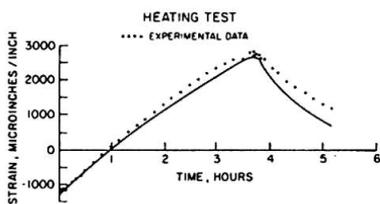
FIG. 3 COMPARISON OF EXPERIMENTAL DATA TO CALCULATED STRAINS
