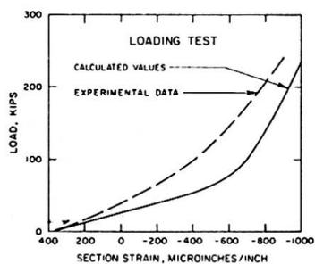
FIG. 4 COMPARISON OF EXPERIMENTAL DATA TO CALCULATED STRAINS
