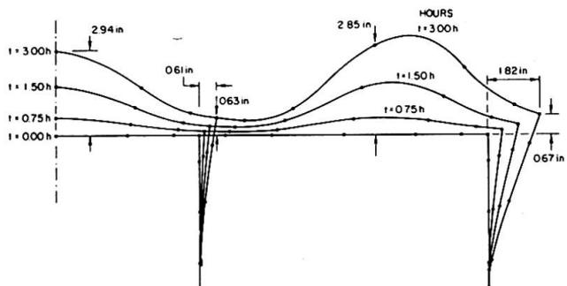
FIG. 8 FRAME DEFORMATIONS
