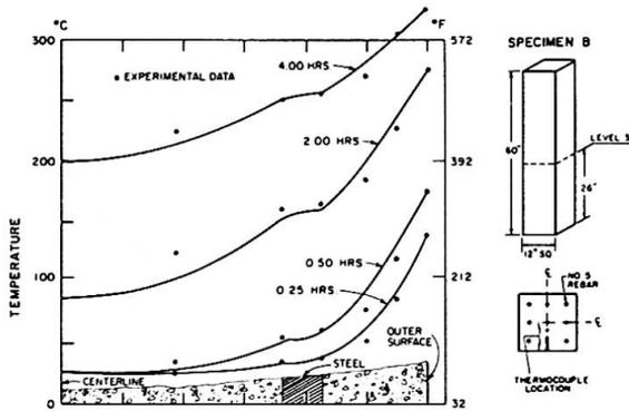
FIG. 2 COMPARISON OF EXPERIMENTAL DATA TO CALCULATED TEMPERATURES
