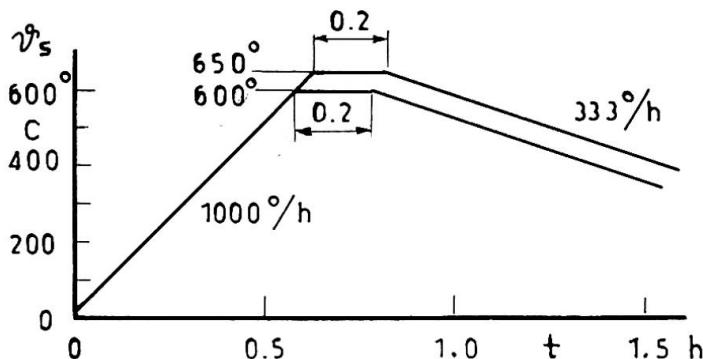
and  $650^{\circ}\text{C}$ . Using the same column section as before, the slenderness ratio  $\lambda = 45$ , the stress was varied to allow interpolation of the value just causing collapse during a temperature cycle. These stresses are also plotted in the diagram, Fig 5.
