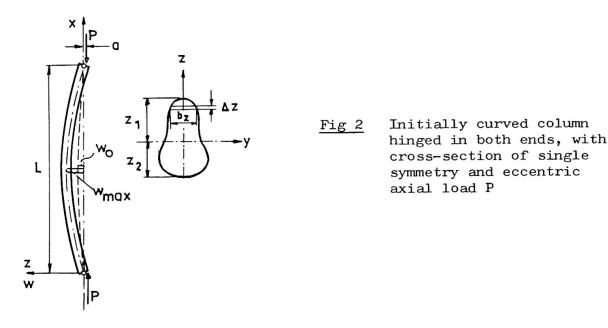
a bending moment will occur increasing the deflection to  $w_{max}$ . If the load is much smaller than the short-time buckling load, and no bending out of the xz-plane can take place, the increase is rather small but if the load is kept constant and creep sets in, the deflection increases with time. The creep strain rate at a distance z from the CG-axis of a section, Fig 2, may be written
