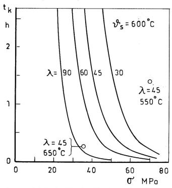
Creep buckling time versus compression stress for various
