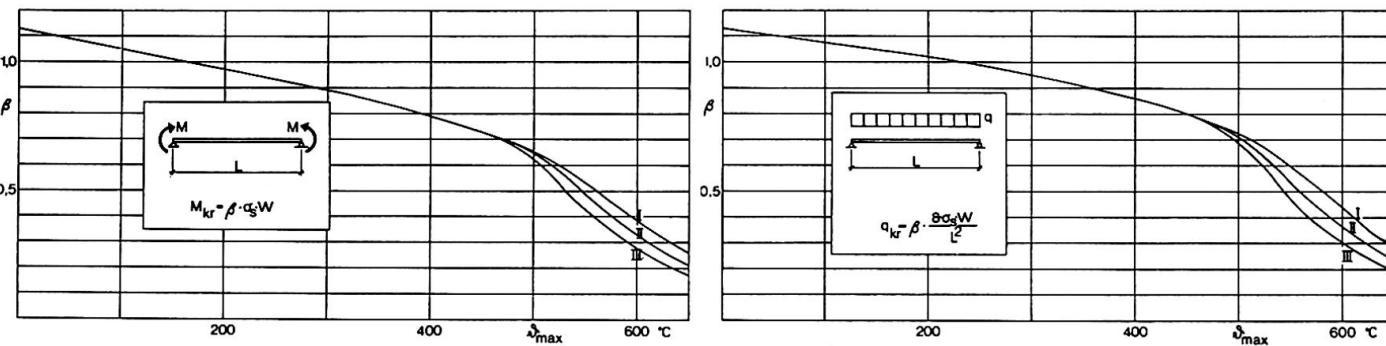
Fig. 3. Load-bearing capacity ( $M_{kr}$ ,  $q_{kr}$ ) for two types of loading at a simply supported steel beam of constant I cross section. Curves I, II, and III correspond to a rate of heating of 100, 20, and  $40\text{C} \cdot \text{min}^{-1}$ , respectively, and a rate of subsequent cooling =  $1/3$  of rate of heating.
