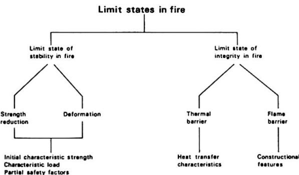
Figure 4 Limit states in fire for structures
