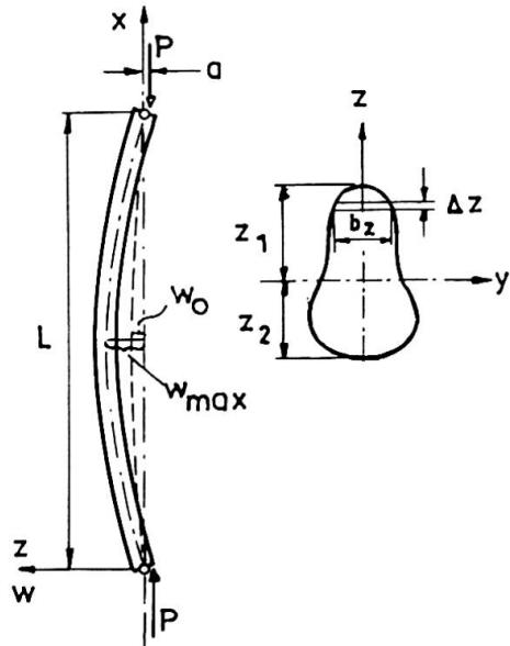
Fig 2 Initially curved column hinged in both ends, with cross-section of single symmetry and eccentric axial load P
