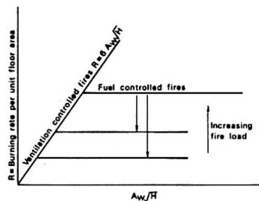
Figure 2 Burning rates of fully developed fires
