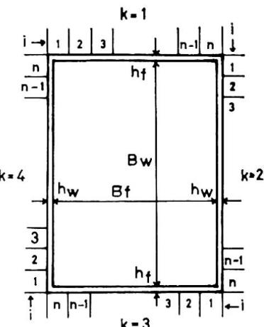
Fig. 2 Mathematical model of cross section of a member
