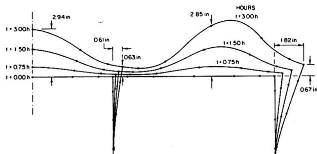
FIG. 8 FRAME DEFORMATIONS
