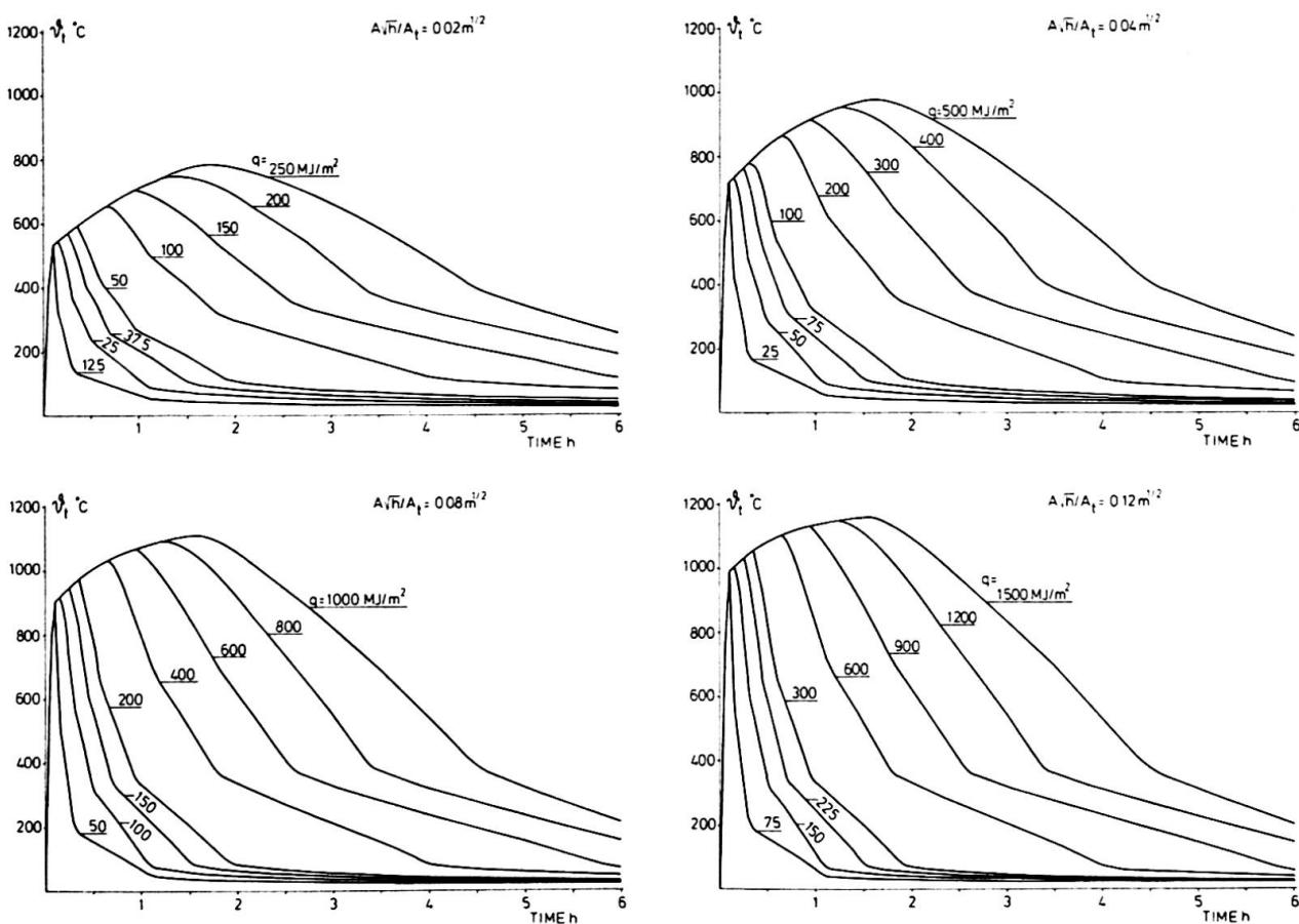
Fig. 2. Gastemperature-time curves  $\vartheta_t$  of the complete process of fire development for different values of the fire load density  $q$  and the opening factor  $A\sqrt{h}/A_t$ .
