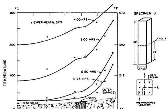
FIG. 2 COMPARISON OF EXPERIMENTAL DATA TO CALCULATED TEMPERATURES
