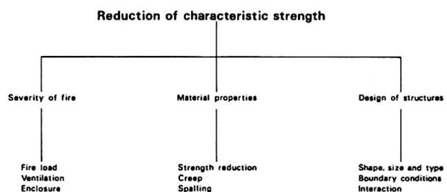
Figure 6 Factors affecting reduction of characteristic strength
