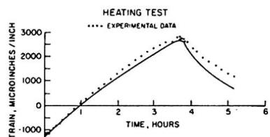
FIG. 3 COMPARISON OF EXPERIMENTAL DATA TO CALCULATED STRAINS
