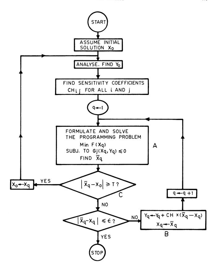
FIG.1. FLOW CHART FOR THE OPTIMIZATION PROCESS
