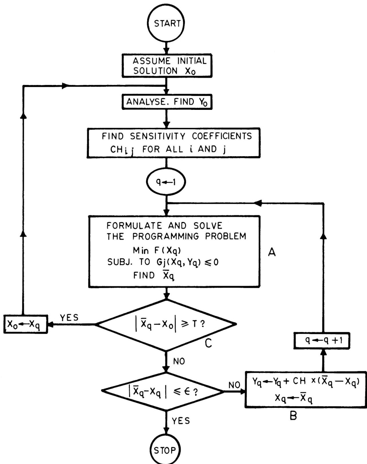
FIG.1. FLOW CHART FOR THE OPTIMIZATION PROCESS
