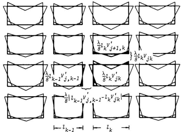
Fig. 7 Decomposed Moment Diagram for Gravity Loads
