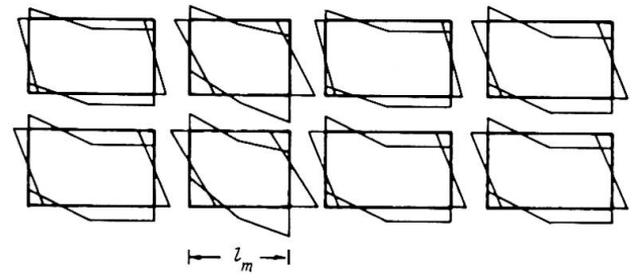
Fig. 6 Frame moments under the wind load (-PWj)
