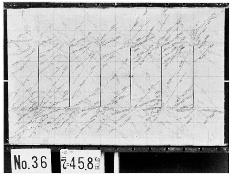
(a) Crack pattern in a Slitted Test-Wall---When the applied shear force is 45.8kg/cm<sup>2</sup>, the cracks are distributed finely with no major diagonal cracks.
