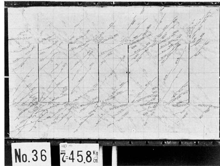
(a) Crack pattern in a Slitted Test-Wall---When the applied shear force is  $45.8\text{kg}/\text{cm}^2$ , the cracks are distributed finely with no major diagonal cracks.
