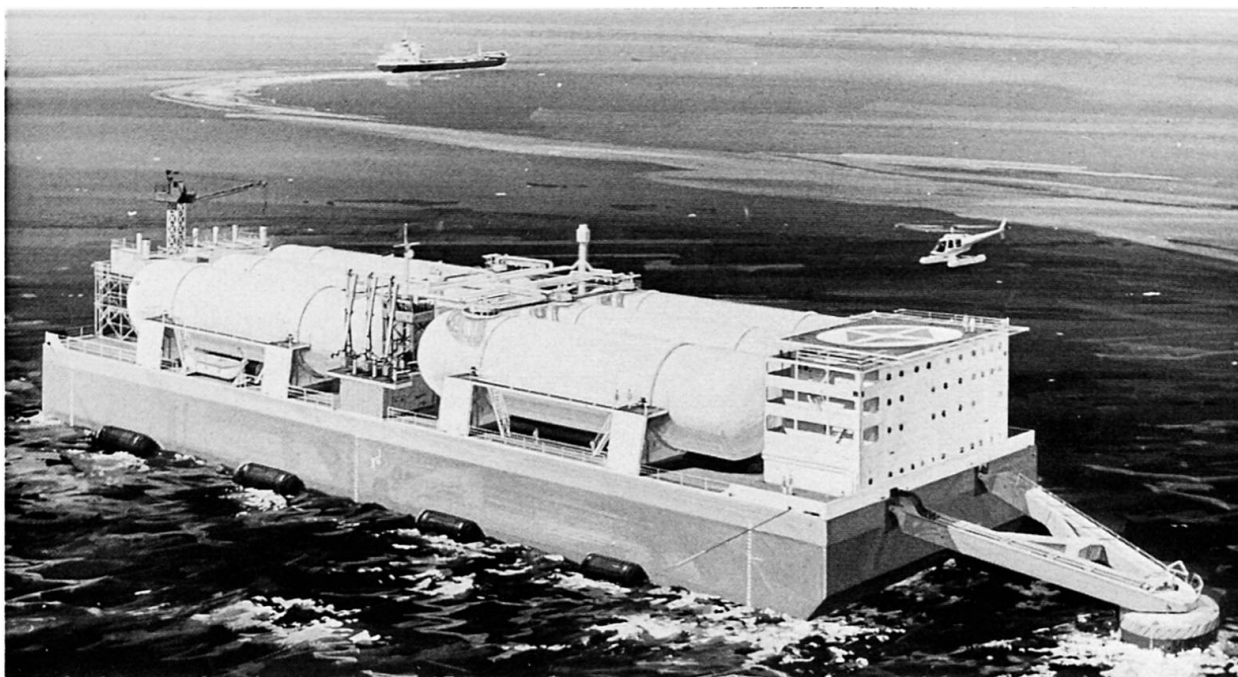
Fig. 13: Liquid petroleum gas production facility, pre-stressed concrete hull. Total displacement 65,000 tons. To be located in the Java Sea.
