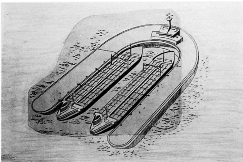
Fig. 12: Concrete floating harbor proposed by Ulrich Finsterwalder.
