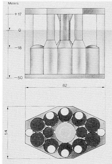
Fig. 12. Dimensions unit shown Fig.11
