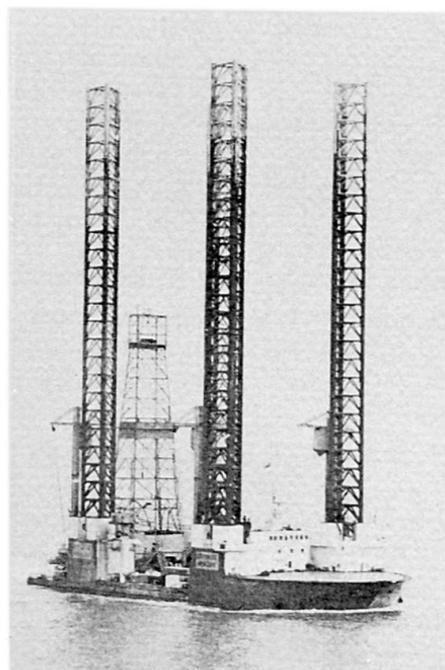
Fig. 3. Self-propelled Jackup
