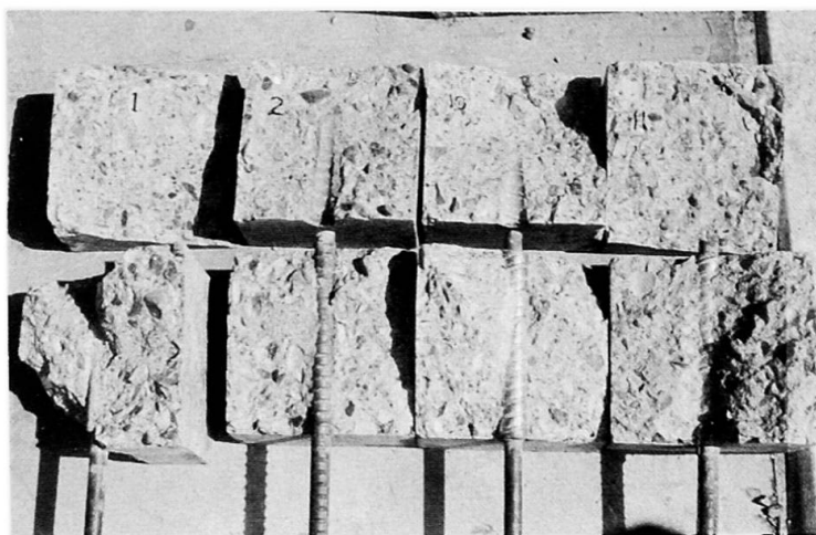
Phot.1 Inside of specimens after pull-out bond test
