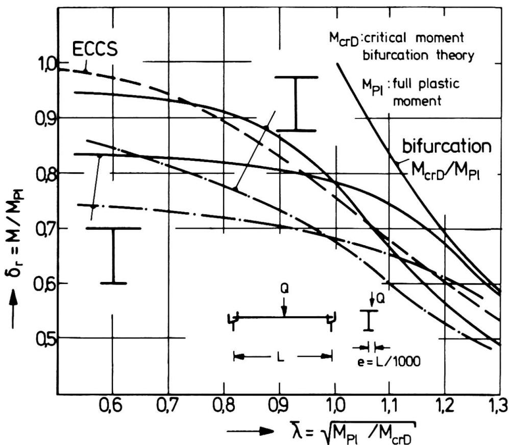
fig.5: load carrying capacity StE 70
