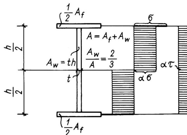
*Fig. 2. Elastic stress patterns for hybrid I-beam; Author's assumption*
