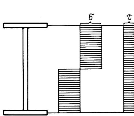
*Fig. 1. Elastic stress patterns for homogeneous I-beam; assumed in [1]*
