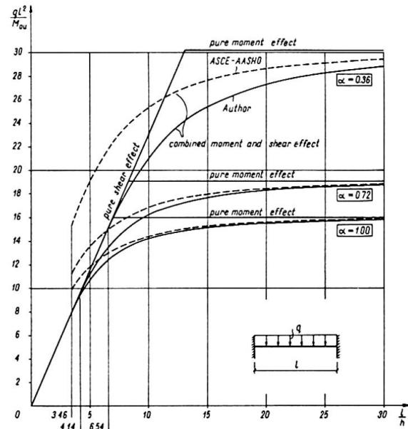
Fig. 5 Collapse loads - uniform
