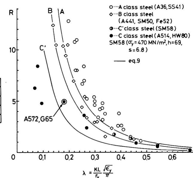
Fig.5 Rotation Capacity under Uniform Moment
