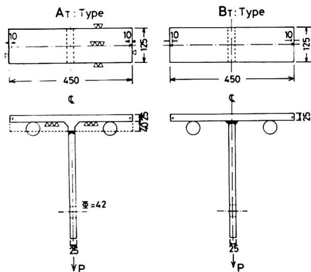
Fig.-6 Specimens of 4-types for bending tests
