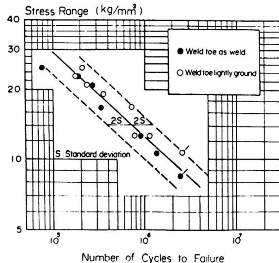
Fig.2 Fatigue Test Results
