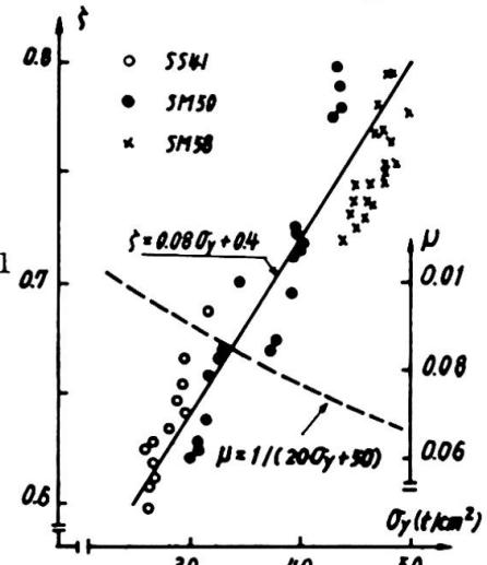
Fig.3 Yield Ratio  $\zeta$  and Strain Hard. Coeff.  $\mu$
