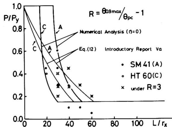
Fig.6 Rotation Capacity of Beam-Columns
