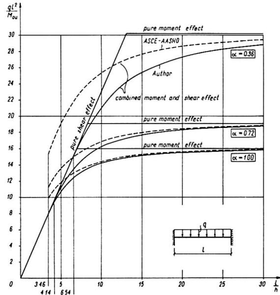
Fig. 5 Collapse loads - uniform
