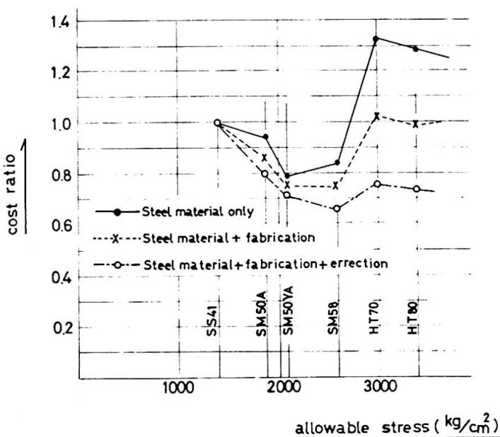
Fig. 1 Relation between allowable stress and cost ratio
