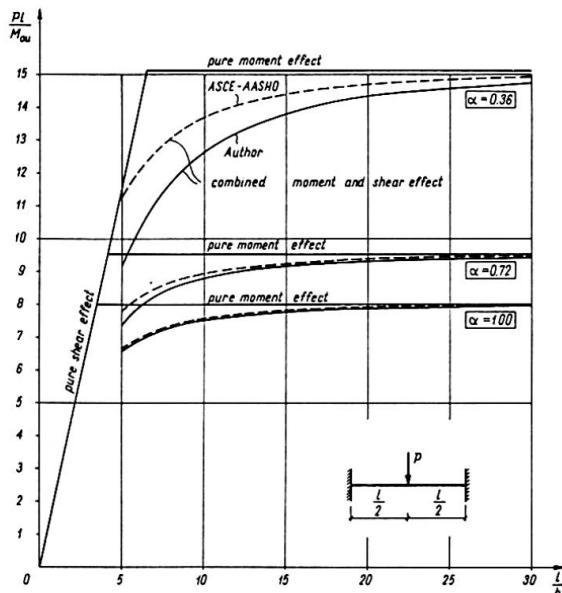
Fig. 4 Collapse loads - concentrated
