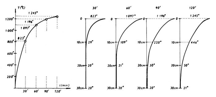
Fig. 5 Calculated temperature history during the fire
