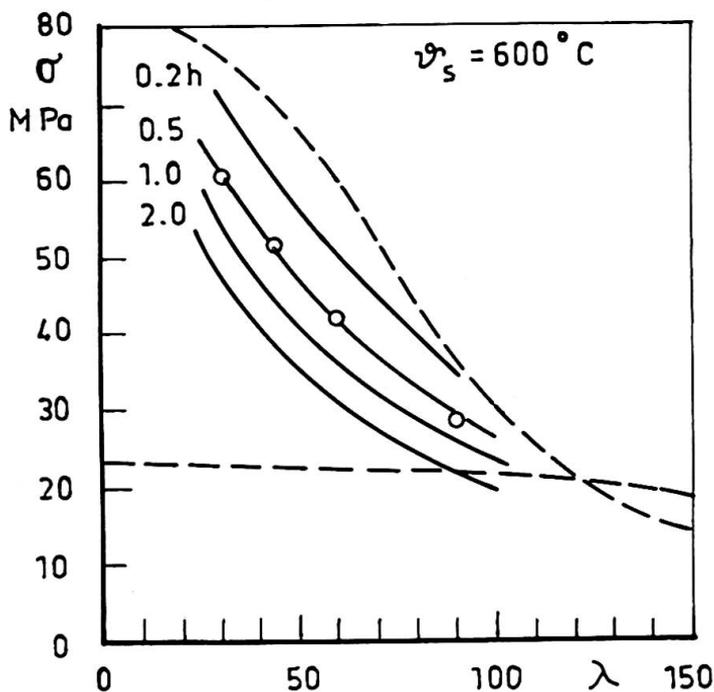
Fig 2 Buckling stress versus slenderness ratio for various times of exposure to 600°C and for temperature-time history with maximum temperature 600°C
