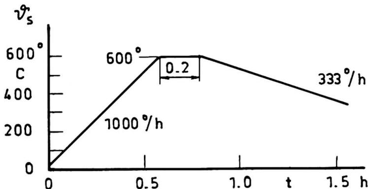
Fig 1 Temperature-time history introduced into computer programme
