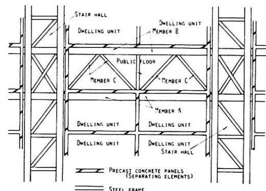
Fig. 2: The fire compartment and steel frame
