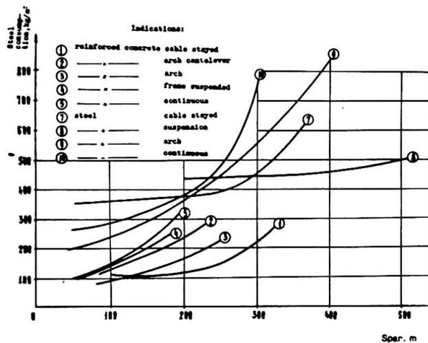
Fig. 6 Relation between steel consumption and span
