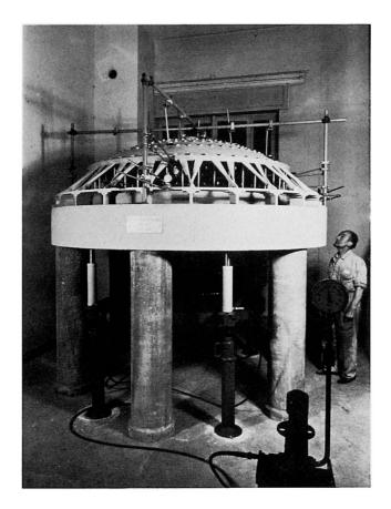
FIG. 1 1:50 scale elastic model of the 130 m dia.cir cular reinforced concrete shell roof of Norfolk Cultur al Center (Virginia, USA). Statical tests.
