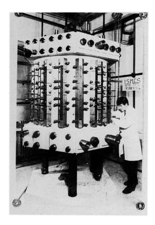
FIG. 3 1:20 scale structural model of the prestress ed concrete vessel of the THTR nuclear reactor.
