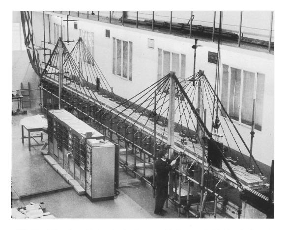
FIG. 10 1:33 scale model of road and railway guyed bridge over the Rio Paranà, Argentina, (complex steel structure). Statical and dynamic tests (running through of a train).
