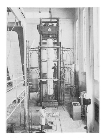
FIG. 7 1:4,7 scale structural model of the main columns carrying the mason ry dome of the Cathedral in  $M_1$  lan. The model is ready for the axial compression test.
