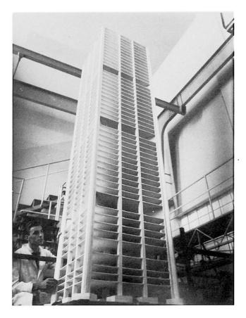
FIG. 5 1:52 scale celluloid elastic model of the 145 m high reinforced concrete building of Place Victoria in Montreal, Canada. Dynamic (seismic) tests.
