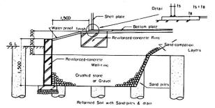
Fig. 10 Example of Improved Detail (2) around the Corner Portion
