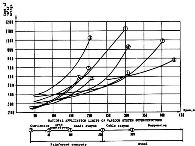
Fig. 8 Relation between cost of 1 m<sup>2</sup> the bridge and span
