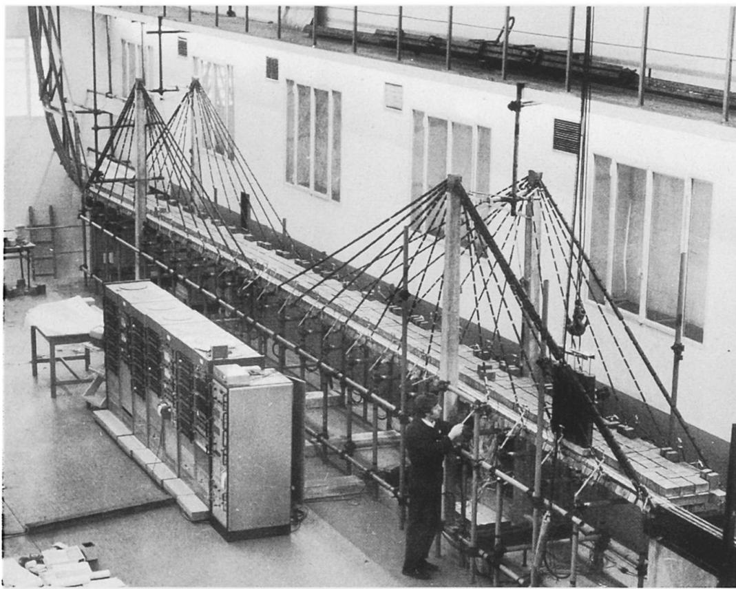
FIG. 10 1:33 scale model of road and railway guyed bridge over the Rio Paraná, Argentina, (complex steel structure). Statical and dynamic tests (running through of a train).
