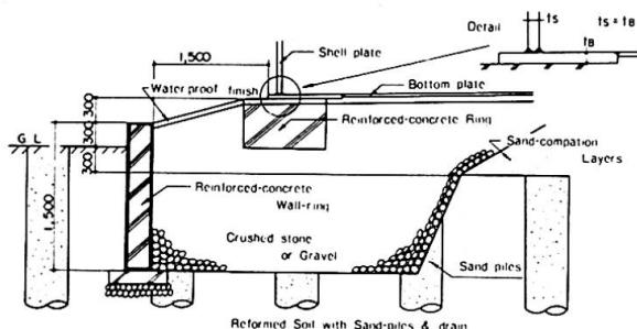
Fig. 10 Example of Improved Detail (2) around the Corner Portion
