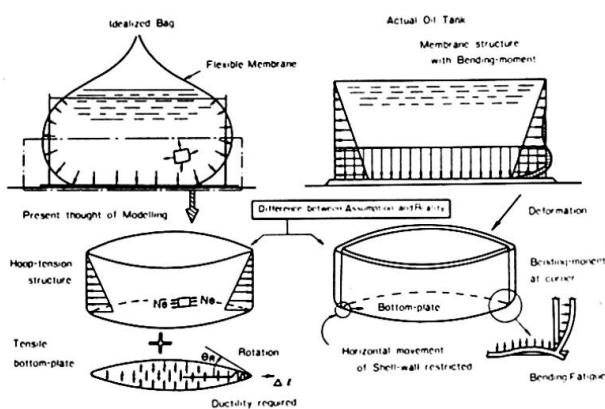
Fig. 2 Structural System and Bottom Plate Deformation Pattern
