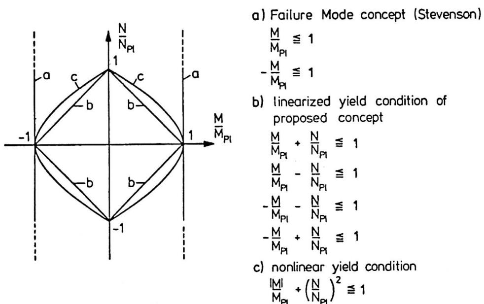
Figure 2 : Yield Conditions of Beam Elements
