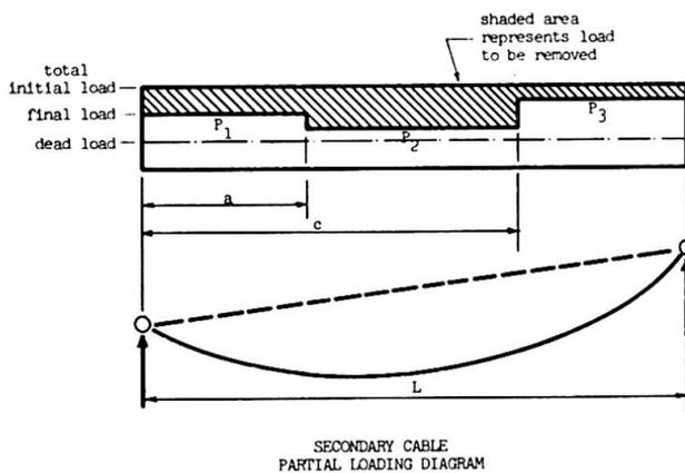
All secondary cables, which were initially of parabolic profile, were replaced by the idealized bar-type elements. The properties of these bar-type elements were determined by equations similar to those previously derived, except that they were generalized to include a set of three partial vertical loads per cable.
