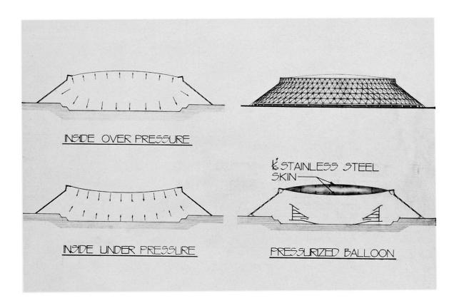
Fig. 3. Stabilization of Metal Skins by Air Pressure.
