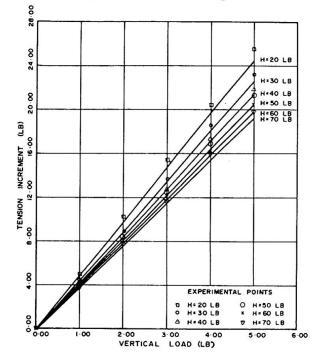
MAX- TENSION INCREMENT IN DOUBLE ROOF MODEL (UNIFORM LOADING)
