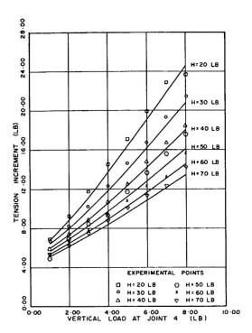
MAX: TENSION INCREMENT IN SINGLE ROOF MODEL (UNIFORM LOAD OF I LB/JT + CONC: LOAD AT THE JT) Fig. 4
