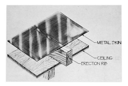
Fig. 5. Erection Detail
