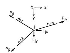
Fig. 1. Force system at a joint
