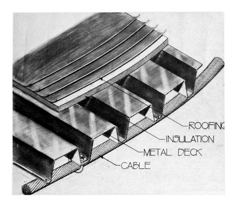
Fig. 1. Conventional Cable Roof Detail
