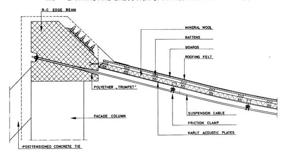
Fig. 4: Section through roof near the edge
