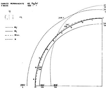
Fig. 8 - Moments and normal forces in the ring for the snow load
