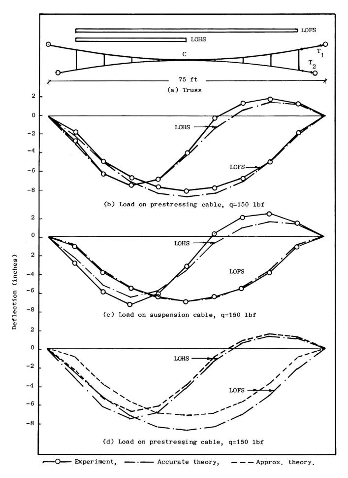
Fig. 2. Deflection diagrams of cable truss
