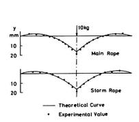
Fig. 5. Deflection curves due to load at mid-span
