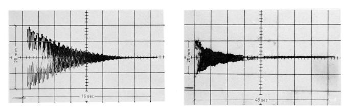
(a) Vibration without cladding, P=150 lbf (b) Vibration with cladding, P=150 lbf Fig. 5.
