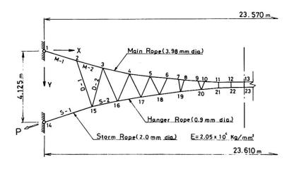
Fig. 4. Cable truss model
