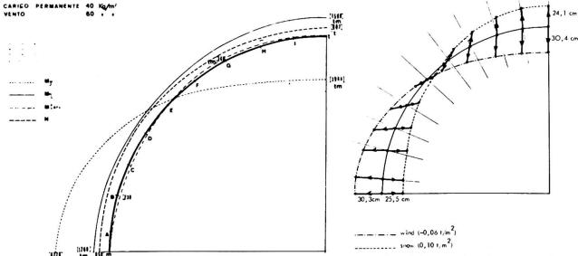
Fig. 9 - Moments and normal forces in the ring for the wind suction
