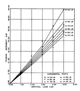
MAX: TENSION INCREMENT IN SINGLE ROOF MODEL (UNIFORM LOADING)
