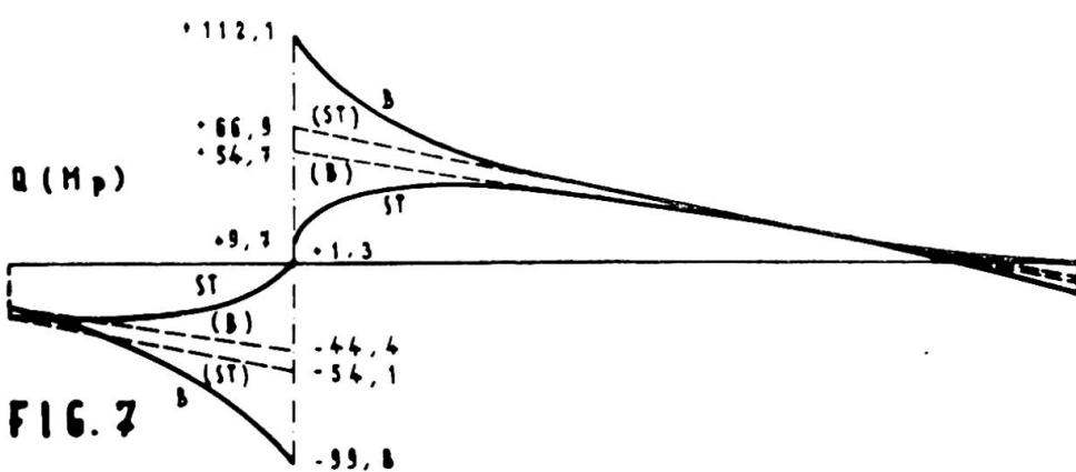
$$\frac{d^2 \psi}{dx^2} = \frac{M}{E J} + \frac{d Q}{G \omega F dx} = \epsilon (M + \beta \frac{d Q}{d x})$$
