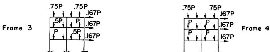
FIG. 2 LOADING CONDITION AT ULTIMATE LOAD
