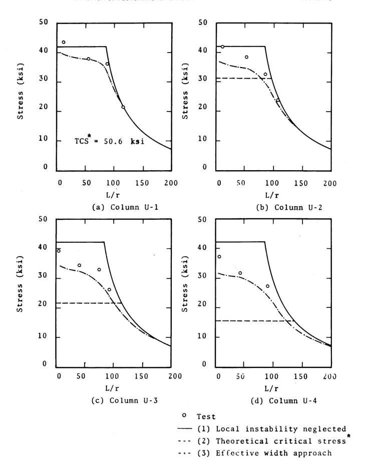
Fig. 4 Comparison of Test Results and Column Curves For Column Specimens U
