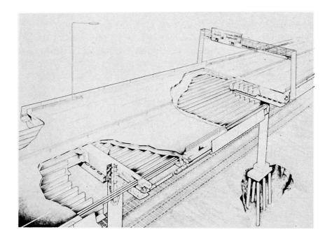
The position of the crosshead columns is variable over a wide range in order to maintain the required clearances from the rail tracks which are not exactly parallel to the road structure.
