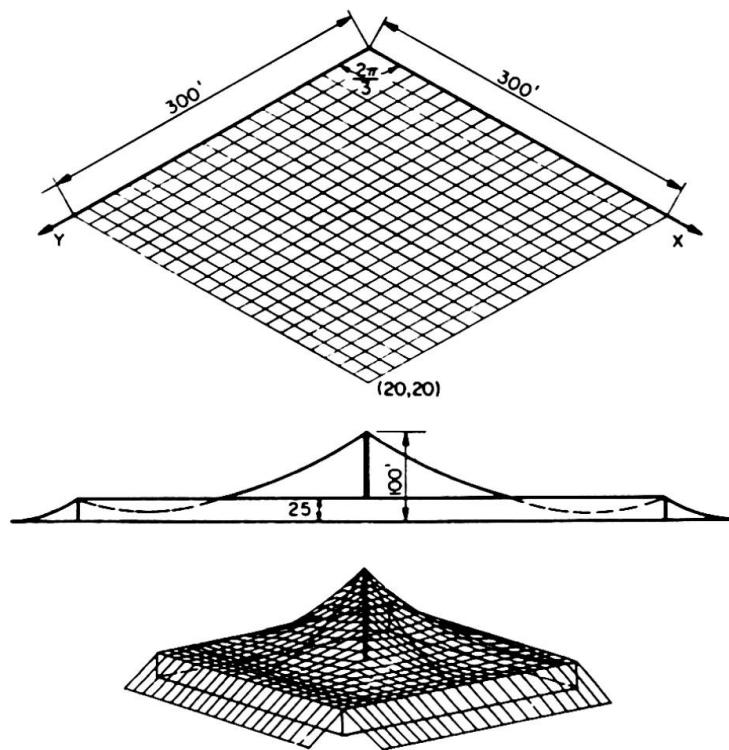
**Fig. 1** Doubly threaded structural net with centre pole
