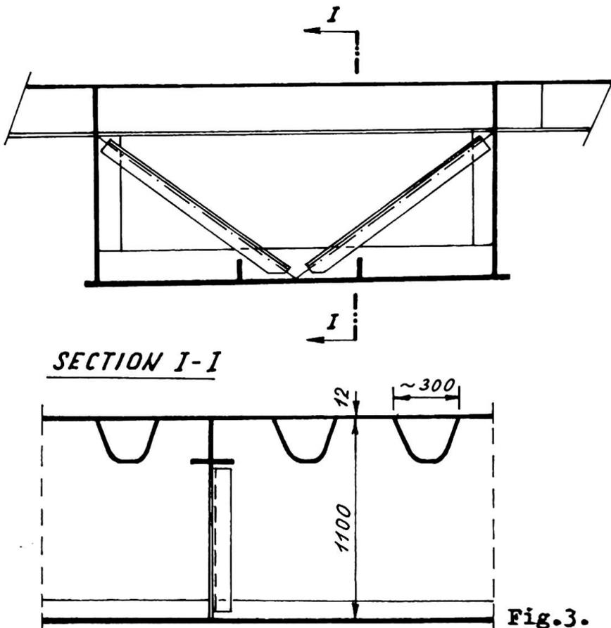
with transverse box stiffeners in trapezoidal shape /fig.3./. Spacing of transverse stiffeners is approximately 600 mm. They rest on webs of main box girders.
