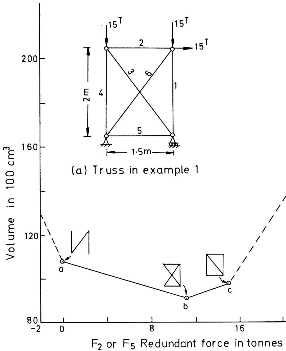
(b) Weight of truss Vs redundant force
