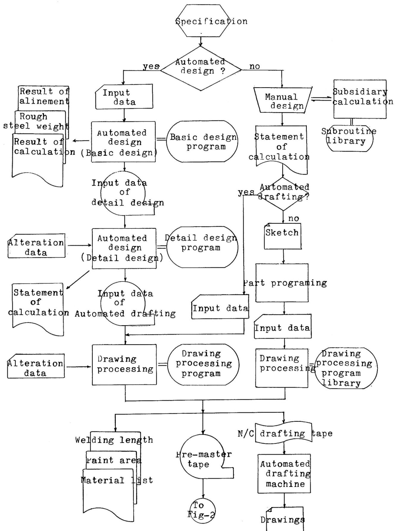
Fig.1 System flow chart of total system (1)
