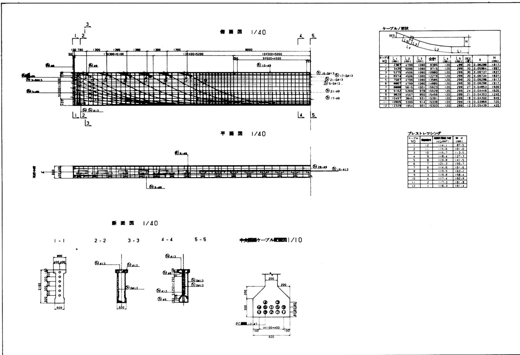
Fig.2 Example of automatic drafting - PC 1 - simple girder
