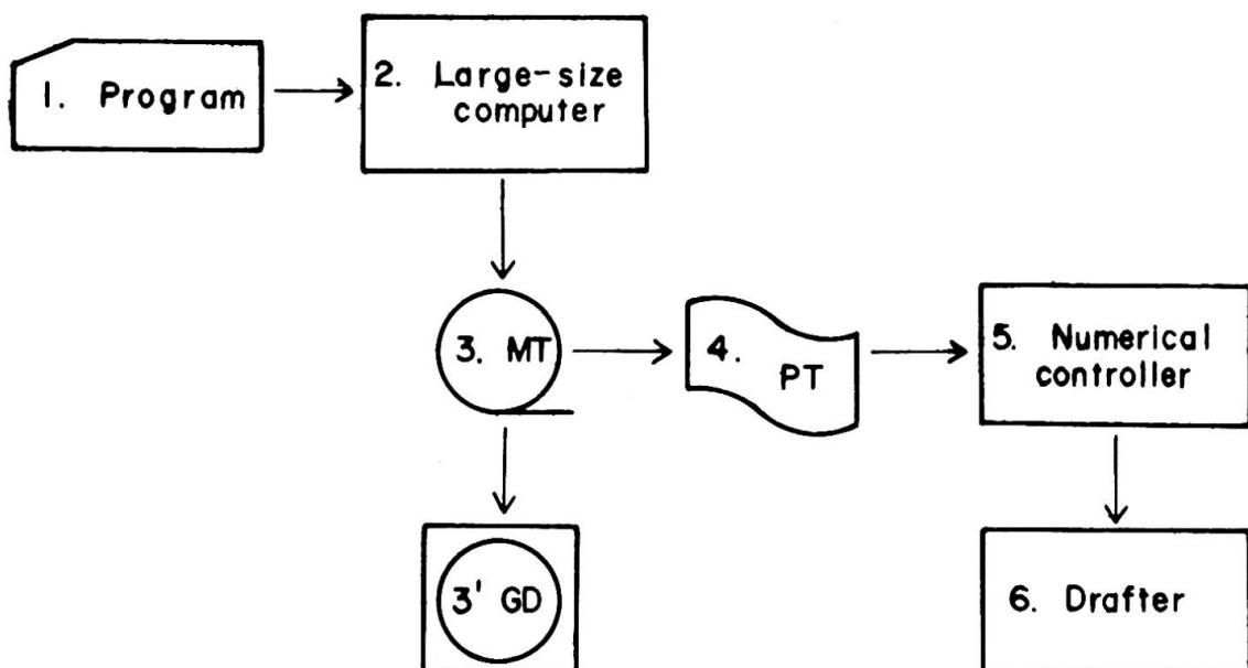
**Fig. 1 Block diagram of automatic drafting process**
