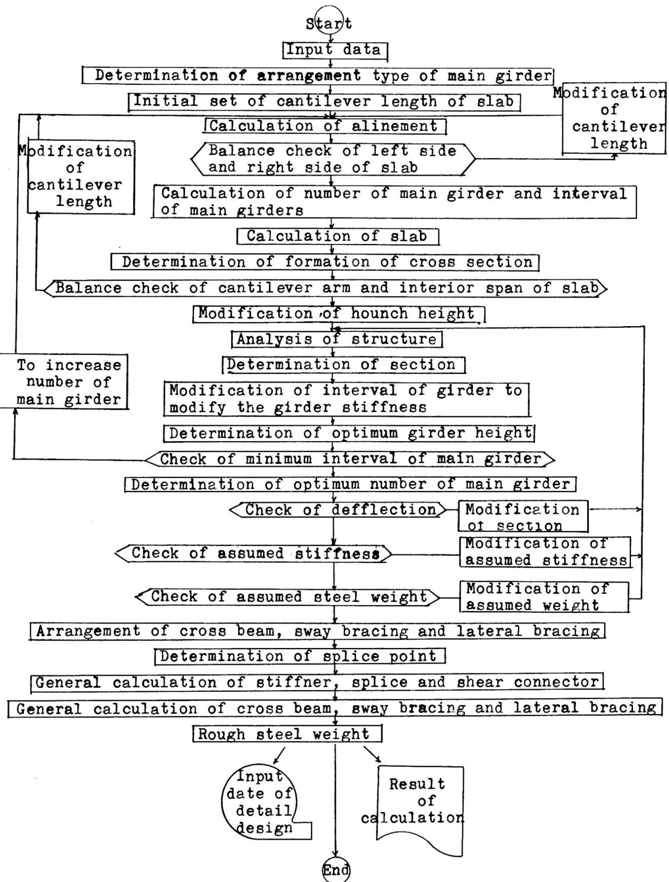
Fig.3 General flow chart of the basic design
