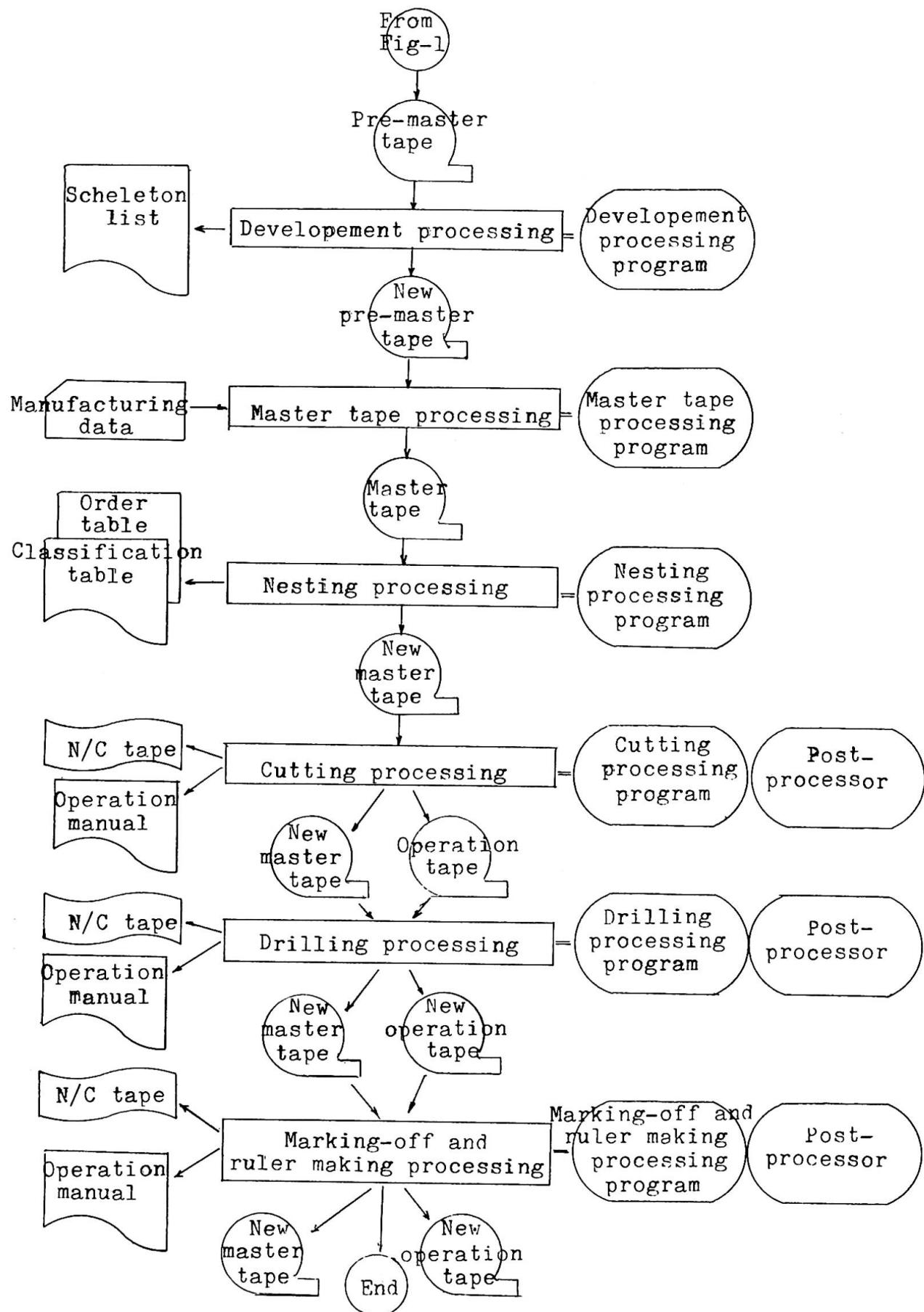
Fig.2 System flow chart of total system (2)
