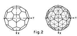
central points of these poligons on the spherical surface and connecting them with the vertexes of the corrispondent poligon, we obtain a triangulated net (fig. 2b) formed by 120+60 isosceles triangols of two types. Now we generate the double-layer spherical shell by four types of different farfallas (differents for side lenght), two of them having one side coincident with a side of two types of
