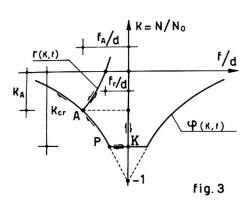
the linear theory of stability and Ā ∓E to elasto-plastic behaviour of material, the deflection f is indeterminate if  $N = N_{cr}$  and  $\Upsilon(M,N) \neq 0$ . When  $\Upsilon(M,N) = 0$  the deflection f is univocally determinate by (1) where we can consider  $M = N f_{\bullet}$  By putting  $d = M_0/N_0$  the (1) can be written:
