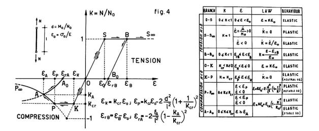
Then the structural analysis can be performed, for each load increment, by the definition of the corresponding behaviour of every bar depending on the position of the representative point in the diagram of fig. 4. This procedure, repeated for successive finite load increments, leads to the evaluation of the collapse-load.
