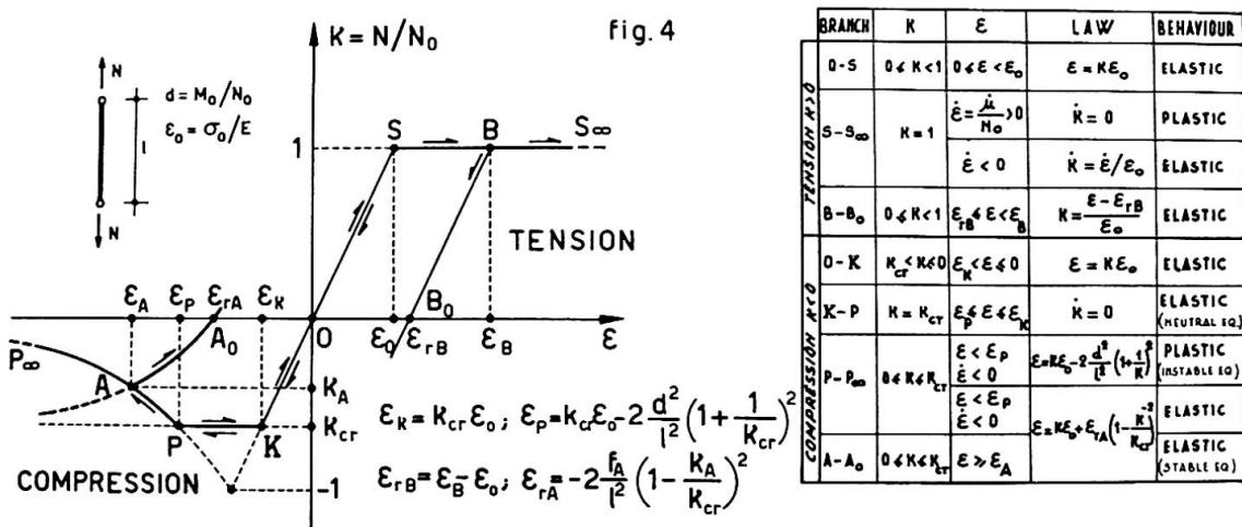
Then the structural analysis can be performed, for each load increment, by the definition of the corresponding behaviour of every bar depending on the position of the representative point in the diagram of fig. 4. This procedure, repeated for successive finite load increments, leads to the evaluation of the collapse-load.
