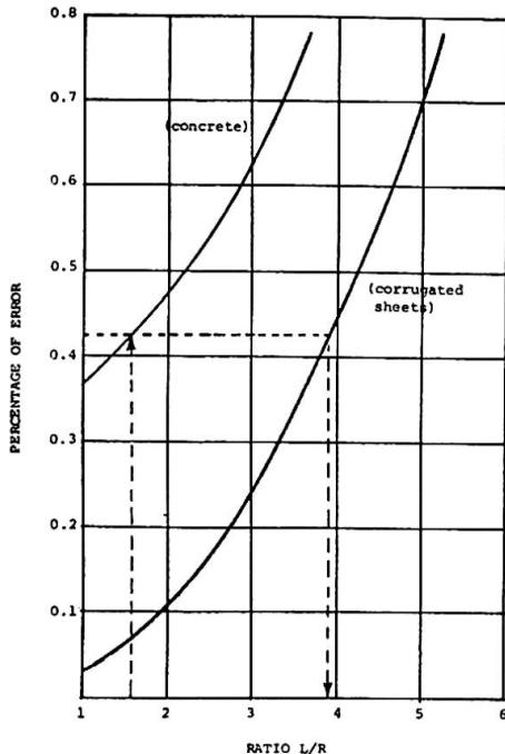
Fig. 2: Percentage of error in roots vs. the ratio L/R
