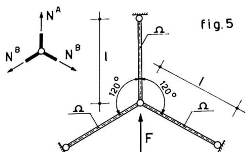
In the elastic field the axial forces are:  $N^A = -2F/3$ ;  $N^B = F/3$ . Being  $|N^A| > |N^B|$  the load increment leads to point K (fig. 4) where is  $\epsilon^A = k_{cr} \epsilon_0$ . The corresponding value of the external force is  $F_K = -1,5 k_{cr} N_0$ . Further external
