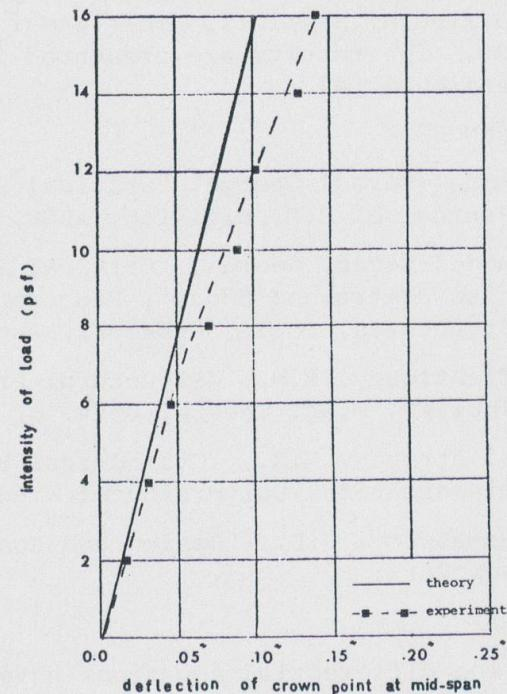
a - COMPARISON BETWEEN THEORETICAL AND EXPERIMENTAL LOAD-
