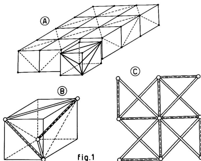
one of which possess a bar shorter than the others, for generating double-layer cylindrical shells (foto 1 top-right).
