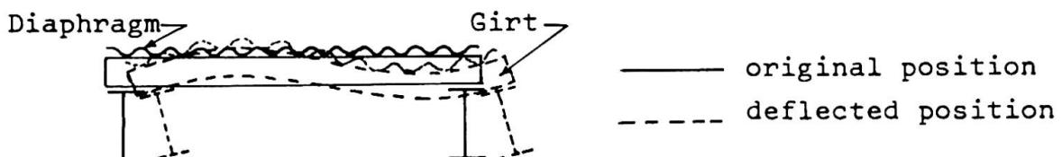
Fig. 4 Columns with Diaphragm-Girt Bracing
