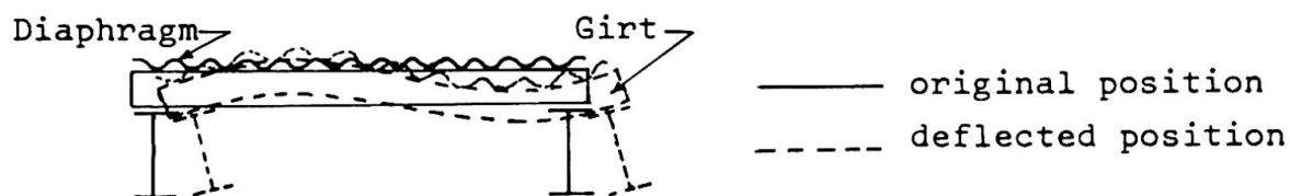
Fig. 4 Columns with Diaphragm-Girt Bracing
