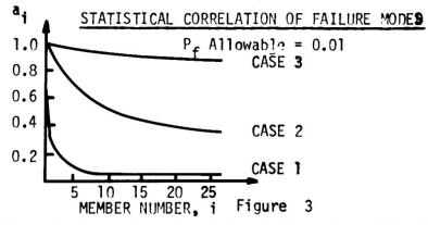
Figure 3 shows the potential weight saving with other frequency distributions and members with unequal lengths and mean applied loads since it indicates the correlation effect and the error introduced into the overall probability expression as the number of members in a structure increases. The magnitude of the weight saving can be obtained from plots of member failure probability vs. member size (or equivalently its safety factor) and is available from the work
