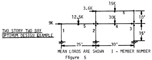
The resulting design moment capacities for the frame in Figure 5 is shown in Table 2 for designs with normal and log normal frequency distribution for load and strength of different coefficients of variation. It is interesting to observe as shown in Table 2 that at least for the examples studied one mode seems to dominate in having a relatively larger failure probability than the other modes. 13
