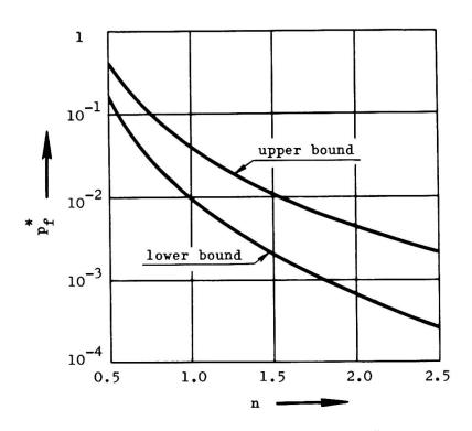
Fig. 1 Probability of Failure  $p_f^{\pi}$  as a function of safety factor n
