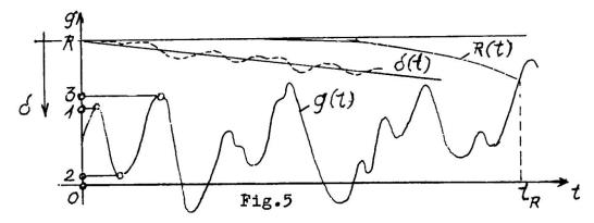
the damage  $\delta$  can be regarded, approximately, as proportional to time and assimilated to a straight line  $\delta = \delta_0 t$ , where  $\delta_0 = \beta \sum_{t=0}^{\infty} |\Delta \sigma|$  is the average damage during a time unit (obtained from the load curve by averaging over a sufficiently long time period). The strength curve is expressed in new units
