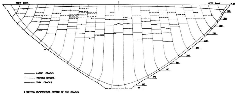
Fig. 7 Flumendosa Dam, Italy. Microcracks on upstream face of model.
